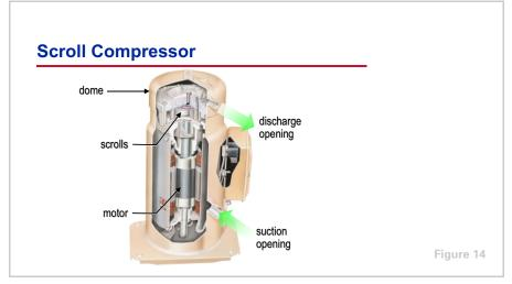
In this example scroll compressor, refrigerant vapor enters through the suction opening. The refrigerant then passes through a gap in the motor, cooling the motor, before entering the compressor housing. The refrigerant vapor is drawn into the scroll assembly where it is compressed, discharged into the dome, and finally discharged out of the compressor through the discharge opening.
